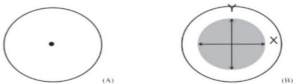
Figure 2: Measurement of inhibition zone diameters (X and Y axes) for Ascosphaera apis fungal growth
